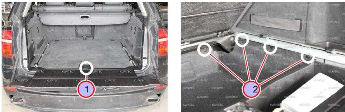
Figure 7: Dismantling the trunk area cladding
