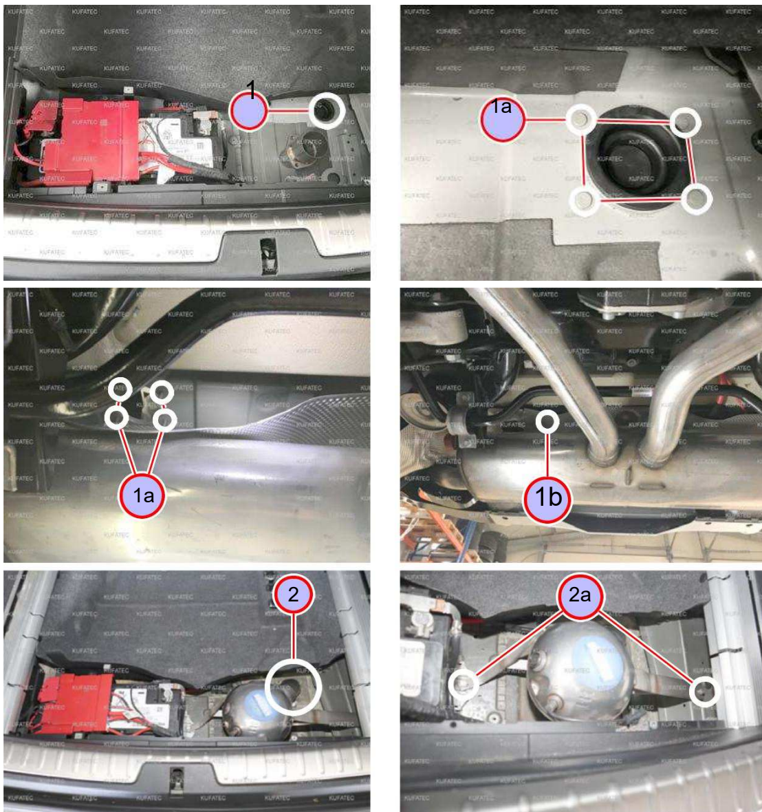
Figure 9: Installation of the noise generator
